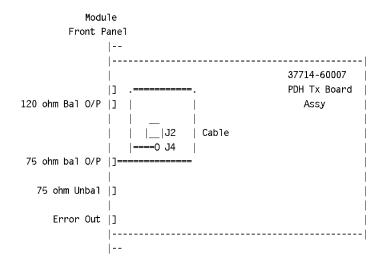
Figure 1 - Showing Preferred Route for cable A7 J4 to Module Front Panel
